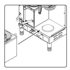
2 Place an empty satellite under the brew basket. Make sure the satellite is pushed all the way back against the front cover.
