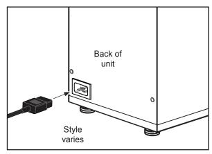
5 Connect the power cord to the appropriate type of electrical outlet.
